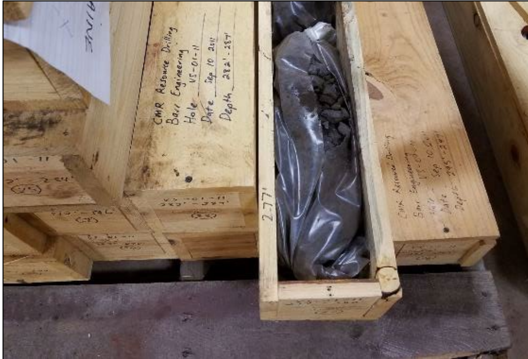
Figure 10-1 Example of Manganese Mineralization. Drill cutting sample from rotasonic drill hole VS-01-11
