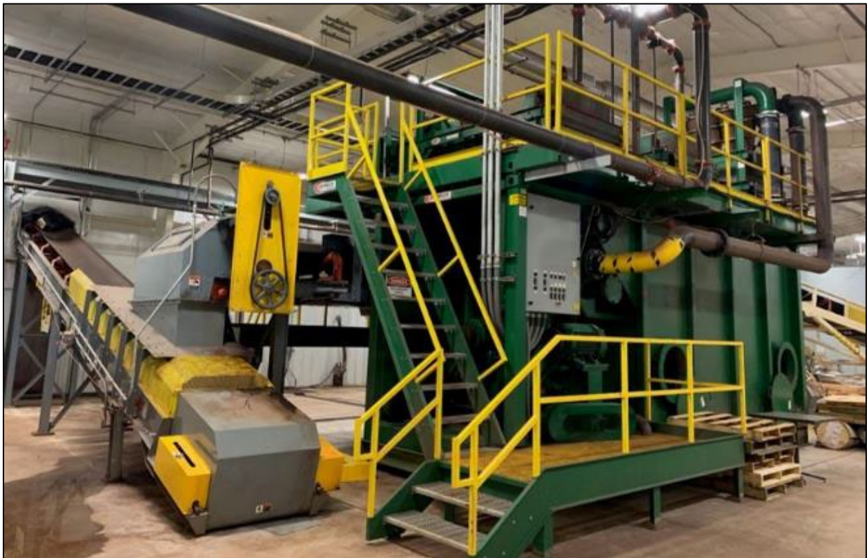
Figure 18-3 Washing and gravity sorting equipment, including conveyors
